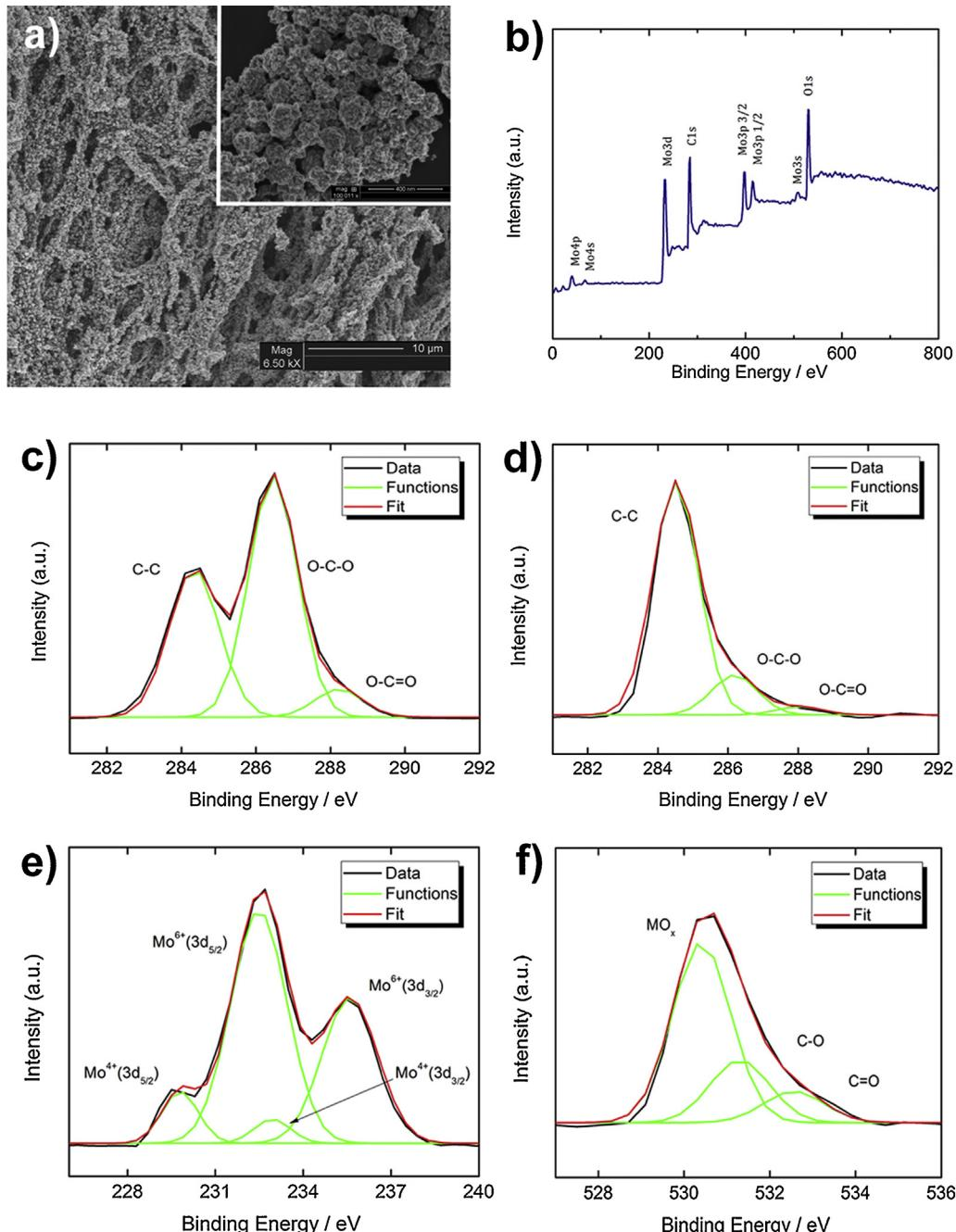
**Fig. 1.** (a) SEM micrograph of RGO/molybdenum oxide hybrid synthesized by the hydrothermal process. The inset shows high magnification image revealing particles of molybdenum oxide on graphene surface. (b) XPS survey spectrum of the hybrid. (c) Deconvolution of C1s high-resolution spectra of the pristine GO. Deconvolution of (d) C1s, (e) Mo3d and (f) O1s high-resolution spectra of the hybrid.
