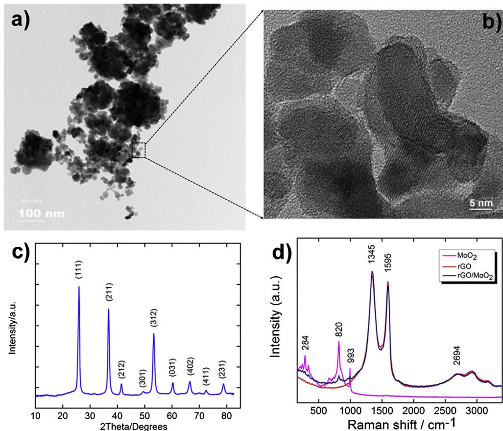
**Fig. 2.** (a) Low- and (b) high-resolution bright field TEM of the molybdenum oxide nanoparticles; (c) X-ray diffraction spectra of the molybdenum oxide. Samples were collected from the bottom on hydrothermal reactor. (d) Micro-Raman spectra of RGO, MoO<sub>2</sub> and the hybrid material.
