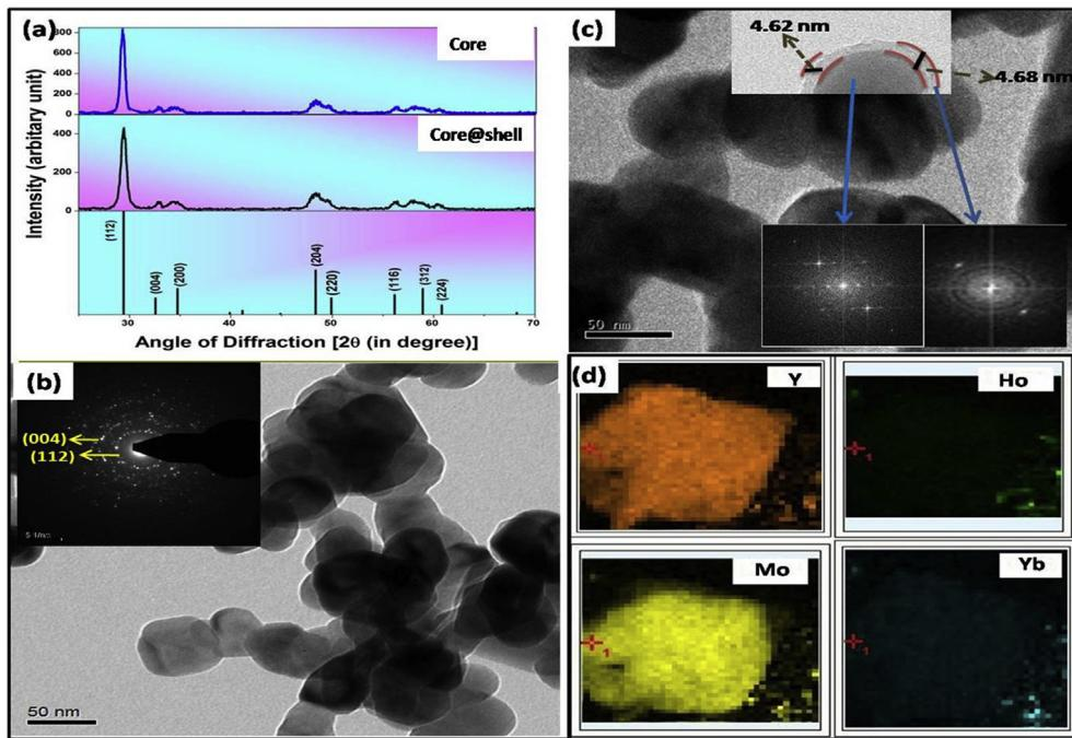
**Fig. 1.** (a) X-ray Diffraction patterns of the core and core@shell nanoparticles, Bright field TEM images of (b) core nanoparticles (inset shows the SAED pattern), (c) core@shell nanoparticles (inset shows the zoom view of the core@shell NPs and the corresponding FFT pattern) (d) The EDS mapping across a particle in the core@shell NPs.
