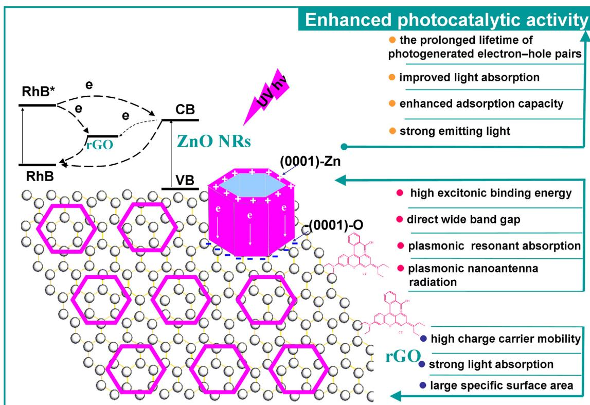
**Fig. 9.** Mechanical illustration of enhanced photocatalytic activity for rGO/ZnO NR composites.
