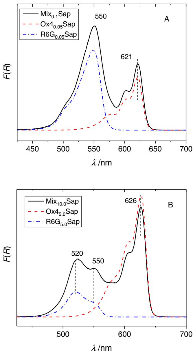
Fig. 1. Absorption spectra of the films prepared from saponite colloids with rhodamine 6G, oxazine 4, or a mixture of the two, with 0.1%CEC (A) and 10%CEC (B) loading.
