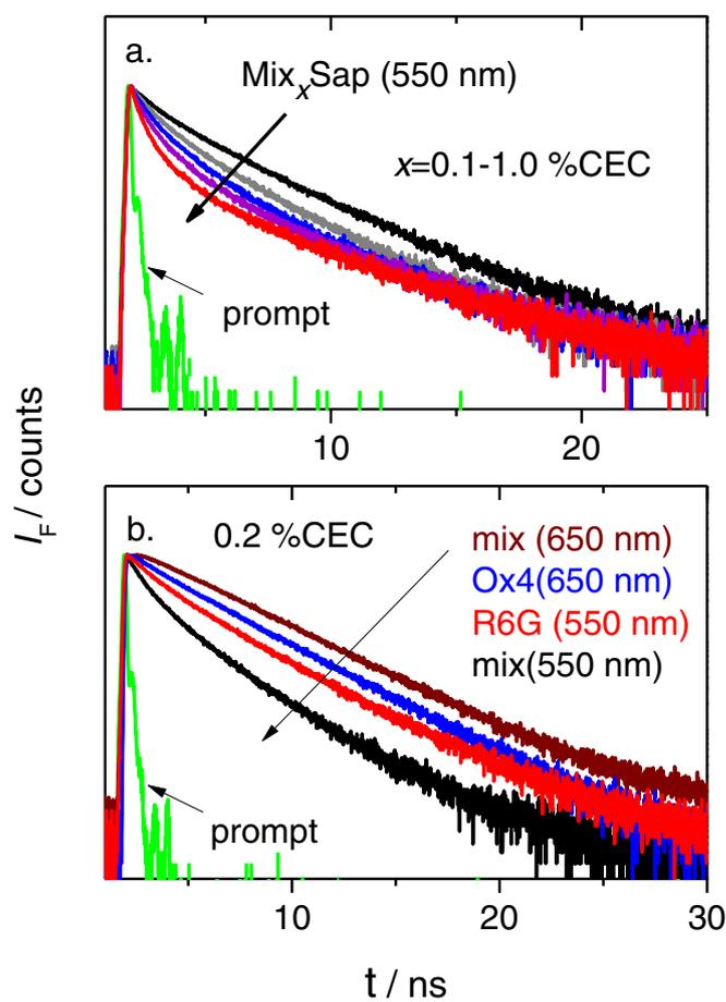
Fig. 4. Time-resolved fluorescence profiles of selected films. a. The effect of dye loading: 0.1, 0.2, 0.35, 0.5, 1.0%CEC. The emission from rhodamine 6G molecules was recorded selectively at 550 nm. b. The profiles recorded at 550 nm were compared for the Mix<sub>0.2</sub>Sap (mix) and R6G<sub>0.1</sub>Sap (R6G) films.
