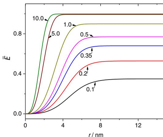
Fig. 6. Calculated values of the theoretical FRET efficiencies and their dependence on the  $r$  value taken as the integration limit.
