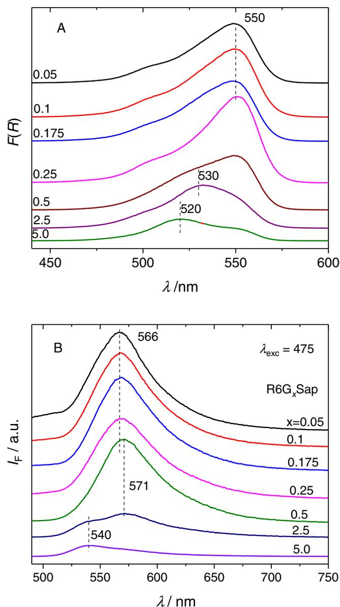
Fig. 2. Absorption (A) and emission spectra (B) of rhodamine 6G/saponite hybrid films with different dye loadings.
