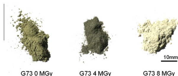
Fig. 6. Photographic image of 75 \mu\text{m} powder samples of glass G73 (0, 4 and 8 MGy). Variation in colour induced by \gamma -irradiation is clearly observed. (For interpretation of the references to colour in this figure legend, the reader is referred to the web version of this article.)
