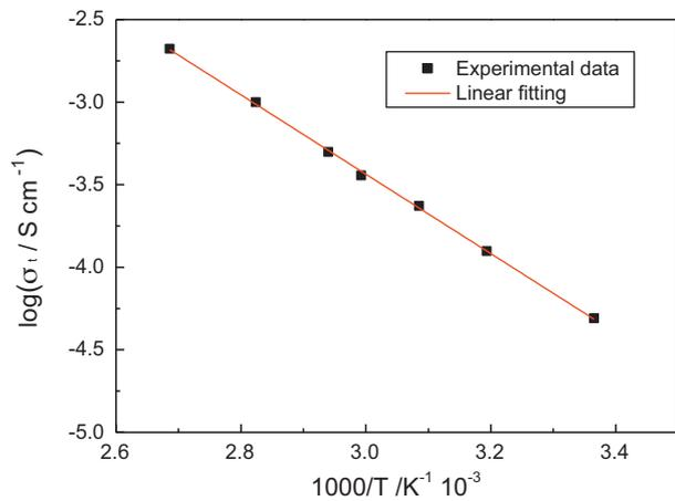
Fig. 4. Arrhenius plot of the total ionic conductivity.
