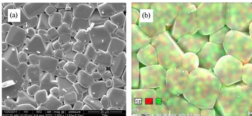
**Fig. 2.** (a) The surface microstructure of the sintered pellet; (b) the mapping image of the elemental analysis obtained by EDS of zirconium (green) and calcium element (red). (For interpretation of the references to color in this figure caption, the reader is referred to the web version of the article.)
