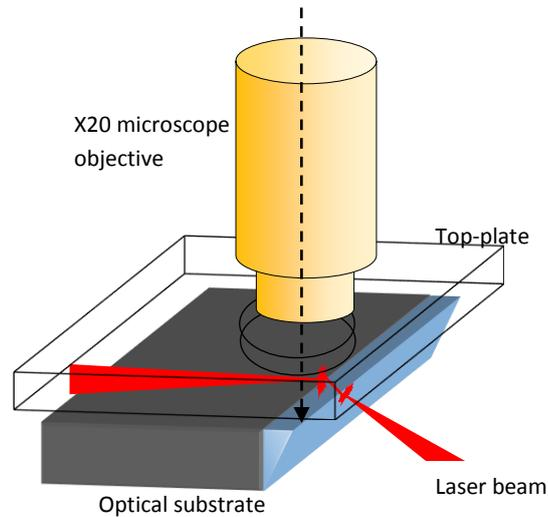
Fig 1.2 Schematic Showing Optical Configuration
