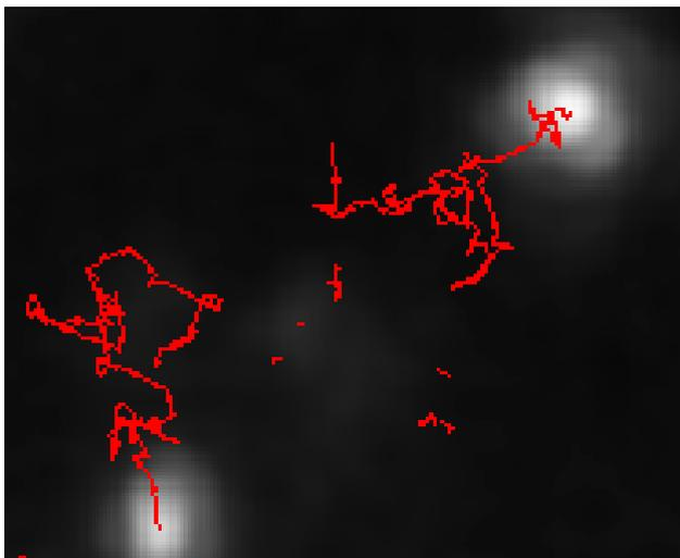
Fig 2. An enlarged image of typical tracks of particles moving under Brownian motion. Note: The image is from the scattered light and is not a resolved image of the particle. Therefore the technique does not provide structural information.
