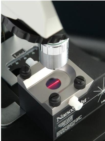
Fig 1.1 Image of Sample Cell
