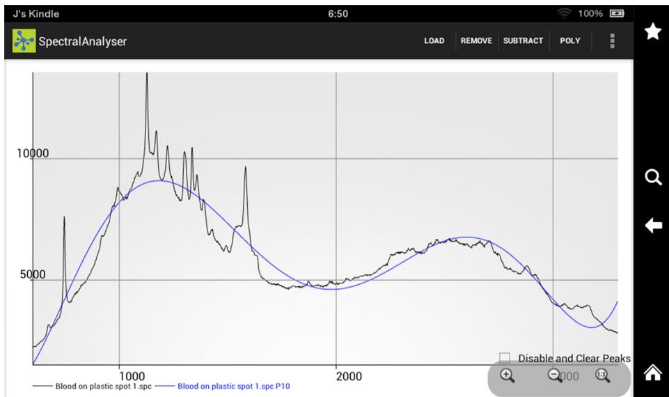
**Fig. 7.** Android App displaying a spectrum and an order 6 polynomial approximation.
