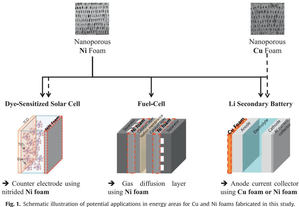
Fig. 1. Schematic illustration of potential applications in energy areas for Cu and Ni foams fabricated in this study.
