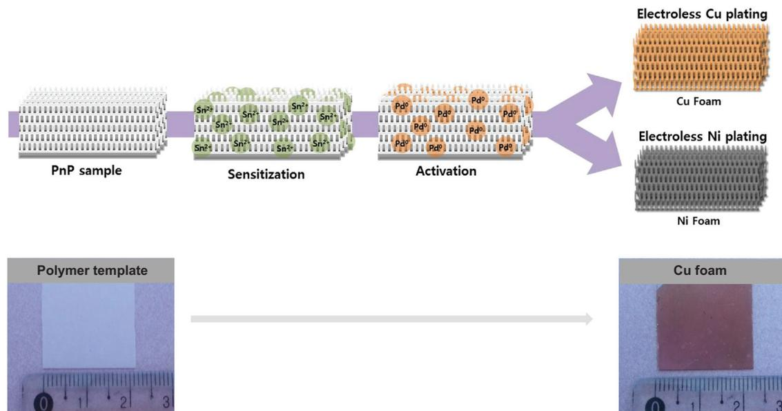
Fig. 2. Schematic illustration of the steps involved in the novel electroless plating method used for the fabrication of Cu and Ni foams with submicron pores. Shown in the micrographs are the pristine polymer template and the polymer template electroless-plated with Cu.
