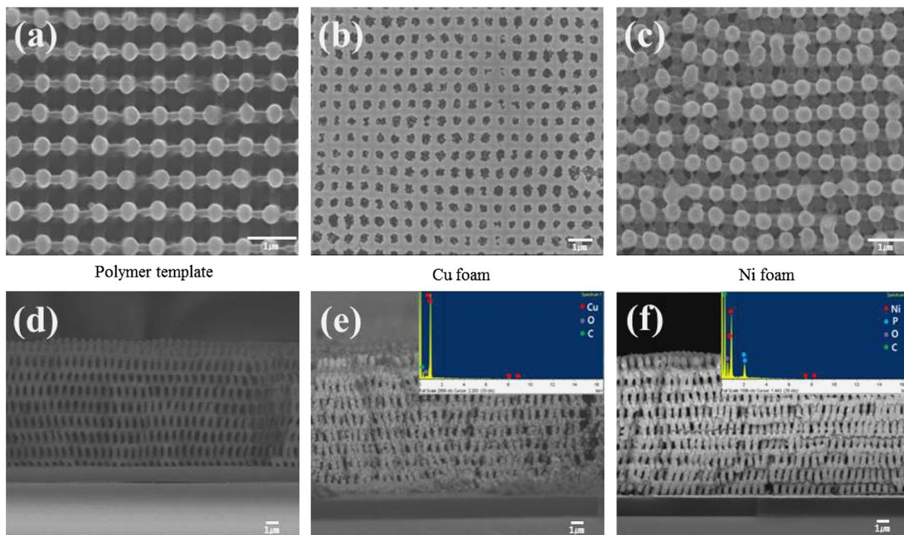
**Fig. 3.** Top and cross-sectional SEM images of electroless-plated Cu and Ni nanofoams: (a, d) PnP polymer template, (b, e) submicron Cu foams, and (c, f) submicron Ni foams.
