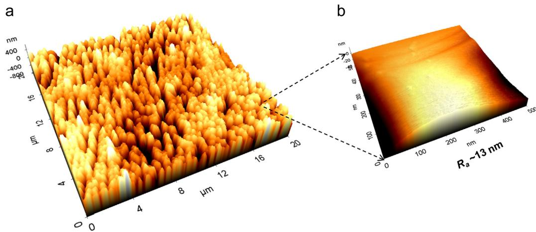
**Fig. 4.** AFM images of (a) the top morphology of the nanoporous Cu foam taken at a low magnification and (b) the smooth surface of a zoomed-in Cu strut with an average surface roughness ( $R_a$ )  $\sim$  13 nm.
