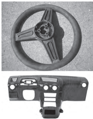
1.11 Schematic of injection moulding (a) and injection moulded wood fibre composite products (b).
