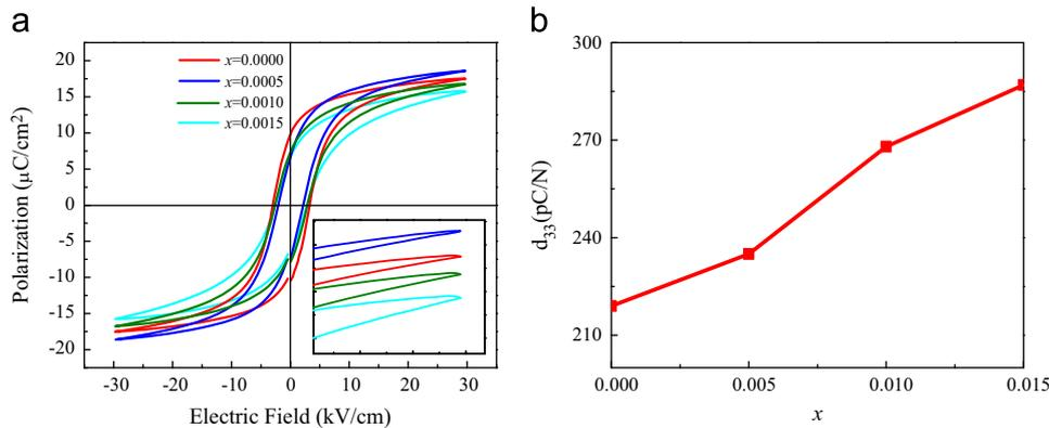
**Fig. 3.** The  $P$ - $E$  loops and the variations of the  $d_{33}$  with  $x$  for the  $\text{Ba}_{0.9}\text{Ca}_{0.1}\text{Ti}_{0.9}\text{Zr}_{0.1}\text{O}_3$ - $x\text{La}$  ceramics with different  $x$  values. (a)  $P$ - $E$  loops and (b)  $d_{33}$ - $x$  curves.
