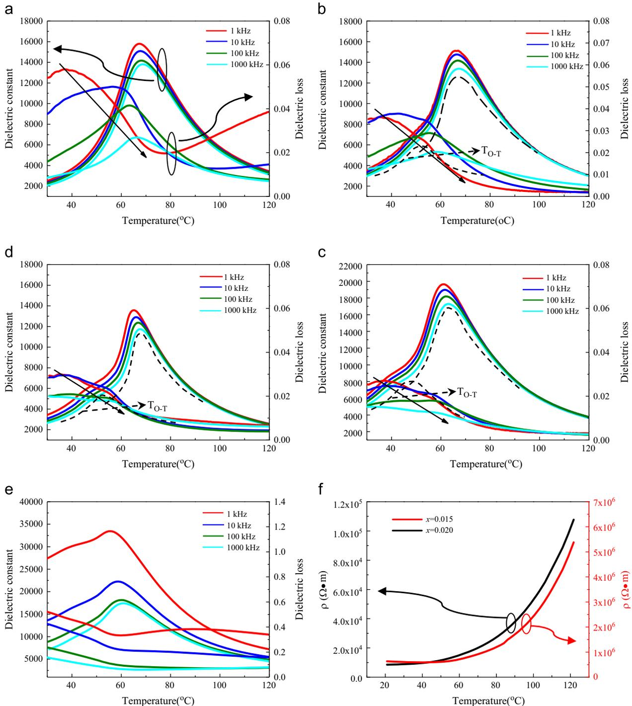
Fig. 2. Temperature dependence of dielectric constant and dielectric loss and the temperature dependence of resistivity for the  $\text{Ba}_{0.9}\text{Ca}_{0.1}\text{Ti}_{0.9}\text{Zr}_{0.1}\text{O}_{3-x}\text{La}$  ceramics with different  $x$  values: (a)  $x=0.000$ ; (b)  $x=0.005$ ; (c)  $x=0.010$ ; (d)  $x=0.015$ ; (e)  $x=0.020$ ; and (f)  $\rho$ - $T$  curves of samples with  $x=0.015$  and  $0.020$ .
