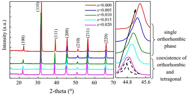
Fig. 1. X-ray patterns of the  $\text{Ba}_{0.9}\text{Ca}_{0.1}\text{Ti}_{0.9}\text{Zr}_{0.1}\text{O}_{3-x}\text{La}$  ceramics with different  $x$  values.
