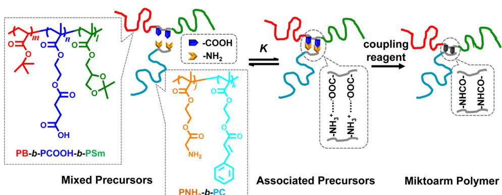
**Scheme 2.** Illustration of the steps involved in the preparation of  $\mu$ -(PB)(PSm)(PC).
