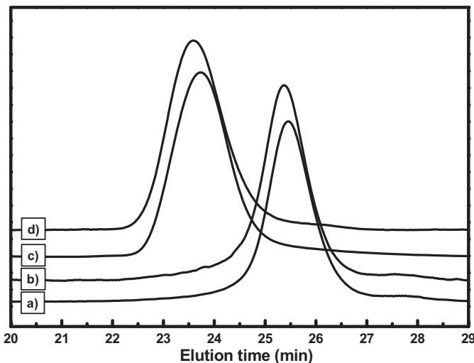
**Fig. 4.** SEC traces of (a) PB-*b*-PHEMA-*b*-PSm<sub>66</sub>, (b) TBC2, (c) PB-*b*-PHEMA-*b*-PSm<sub>200</sub>, and (d) TBC1.
