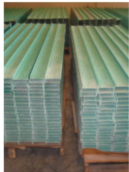
*CBS pultruded composite Egis® studs are tightly packed for shipping to the construction site.*
