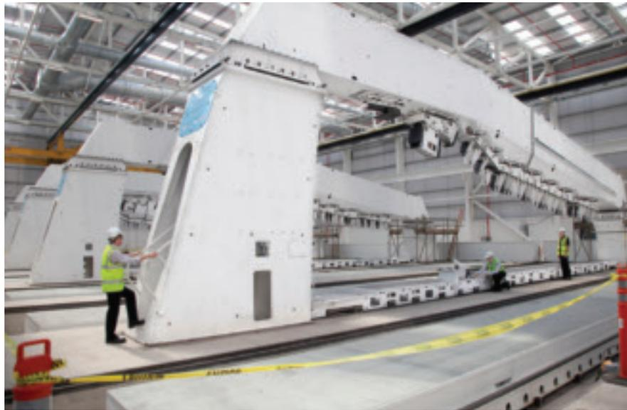
*The semi-automated production jigs being installed as part of Phase 2 activity will enable drilling and other operations to be carried out on CSeries wings.*
