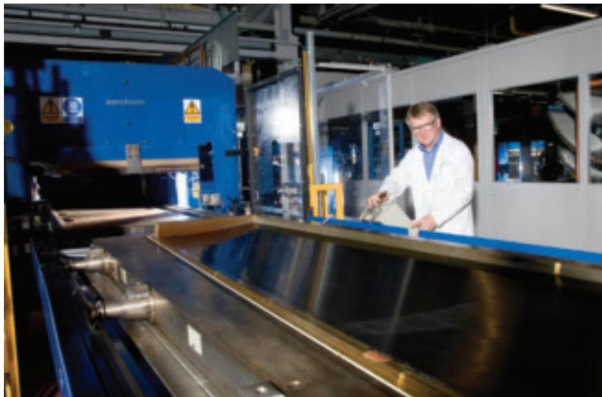
*Bombardier has developed and patented its own resin transfer infusion (RTI) process for the CSeries wing.*
