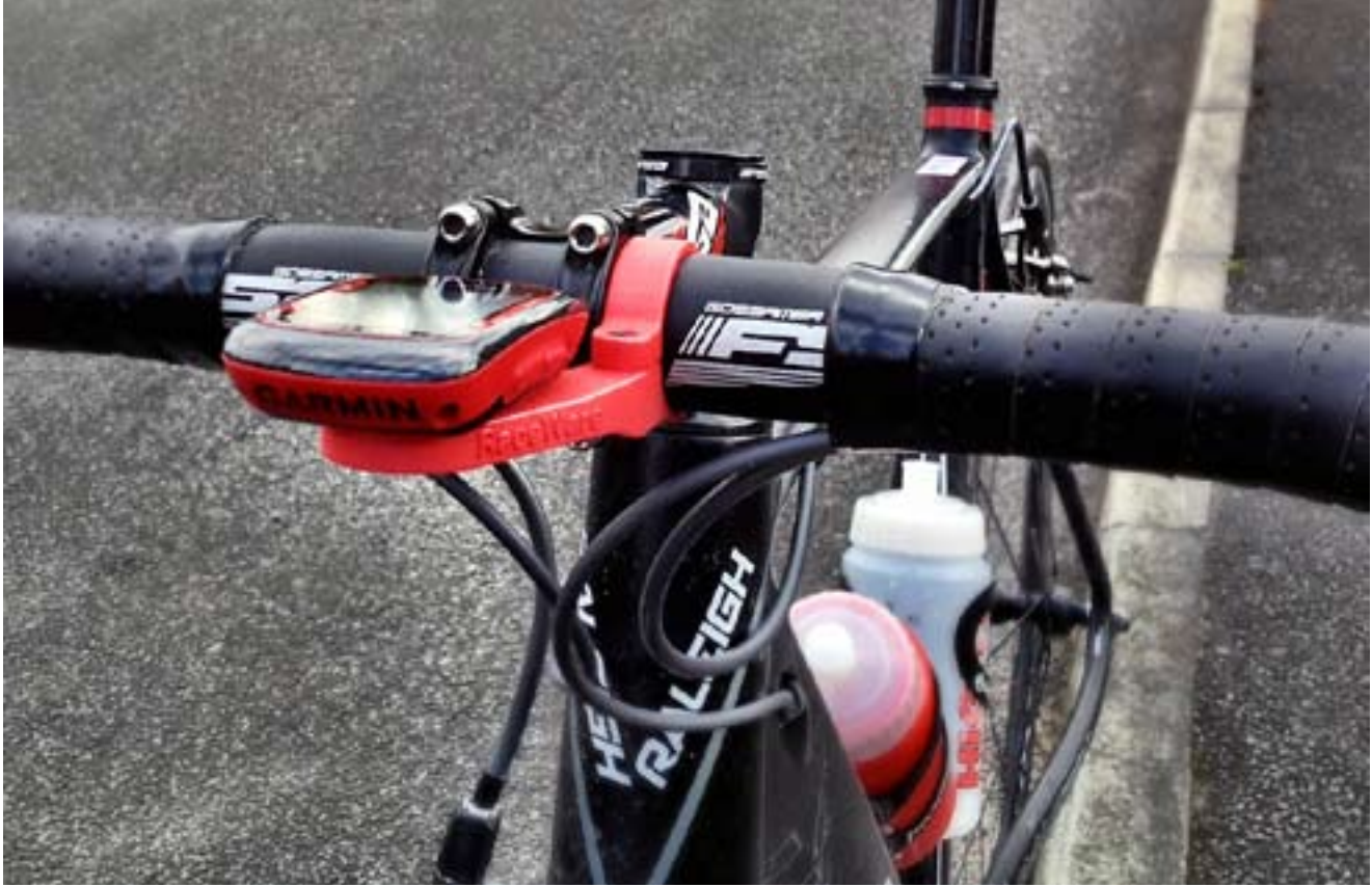
A Garmin GPS computer attached to a road drop bar using a RaceWare mount. The instrument allows a cyclist and his or her team to navigate a route and monitor performance, distance travelled and speed.
