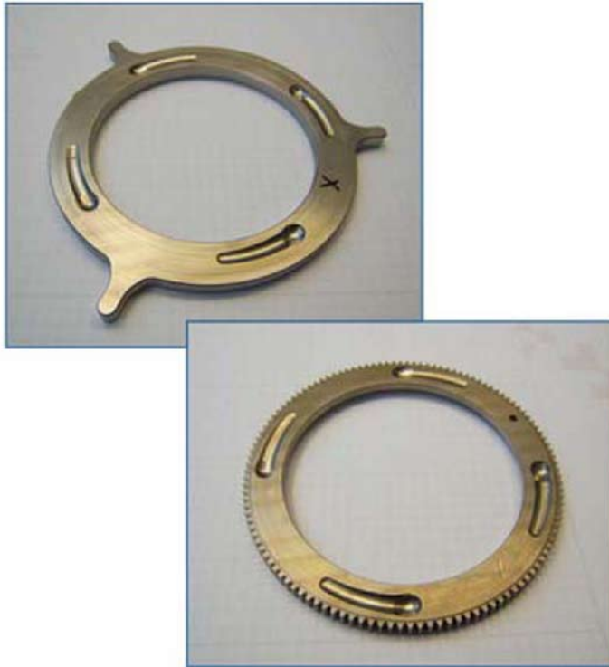
Figure 2. Pressure and activator plates made with lean Cr-Mo PM steels: high-temperature sintered in a roller hearth furnace and accelerated cooling. After Donaldson and Lindsley.
