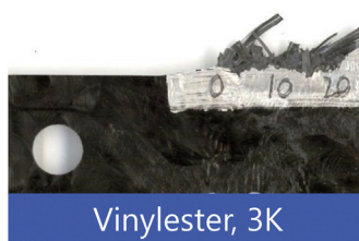
Fracture surface of tow-based discontinuous carbon-fibre composites vs conventional (continuous-fibre) composites: the failure surface of discontinuous composites shows large bundles being pulled-out and broken – meaning that these materials can absorb a large amount of energy as they fail.
