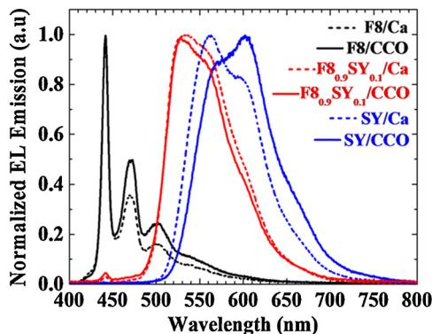
**Fig. 3.** Normalized EL spectra for F8, SY and  $F8_{0.9}SY_{0.1}$  blend PLEDs with CCO interlayer (solid lines) compared with the devices that only have Ca/Al cathode (dashed lines) without interlayer. These EL spectra are shown for devices driven at 4 V.
