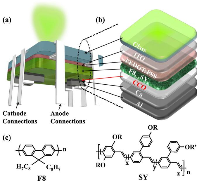
**Fig. 1.** (a) Schematic diagram of F8<sub>1-x</sub>SY<sub>x</sub> ( $x=0, 0.1$  and  $1$ ) based PLED pixels. (b) Different layers in PLEDs. CCO interlayer is used in order to enhance the charge injection in the blend emissive layer. (c) Chemical structure of F8 and SY molecules.
