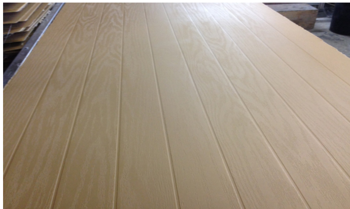
Fine grain feature of finished door surface.
