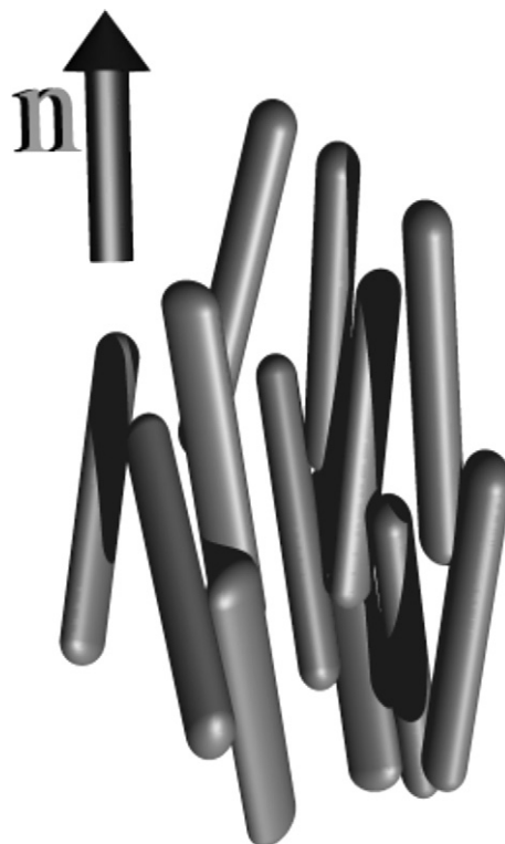
Fig. 1. Cartoon of a nematic phase built from rod-shaped building blocks, drawn with a vertical director n . From [13].
